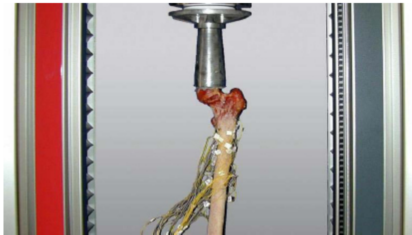
Fig. 9. Test under the load of the human femur [9]
