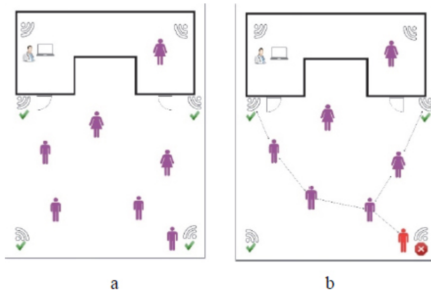
Fig. 13. Variants of medical information system organization based on multiple routers (a) and Mesh network (b).
